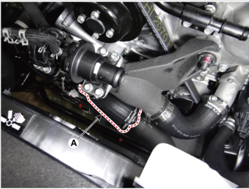
5. Disconnect the oil cooler water hose A (A).
